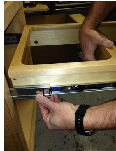
**TIP** By inserting the slides one side at a time, you can be assured that both inner members are properly inserted.
