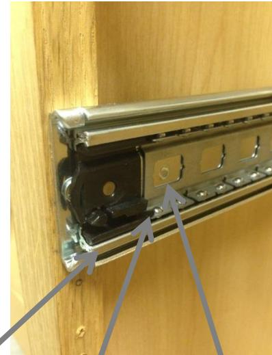
**Step 3** Pull the ball race forward so that it is touching the black plastic guide. Make sure to do this on both slides.
