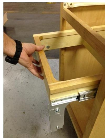
**TROUBLESHOOTING** Inspect the blue plastic mechanism. Make sure there are no gouges in the face. This can be the result of the slides being located too close together. If possible, try to force the slide toward the outside of the floating rear socket.
